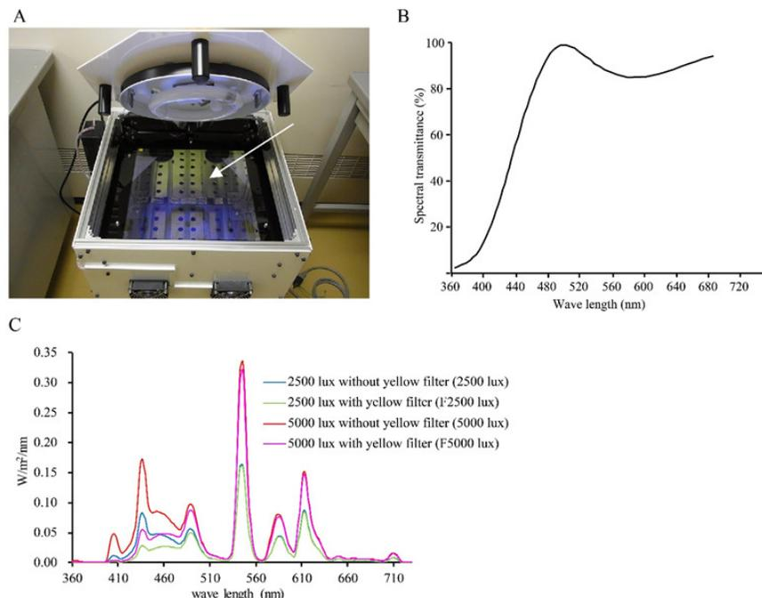
**Figure 1:** Photostress apparatus and spectrophotometric properties of the yellow filter
