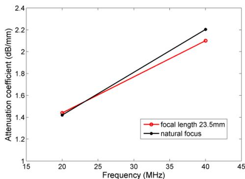
**Figure 6:** Comparison of overall attenuation coefficient between focal and planar transducers
