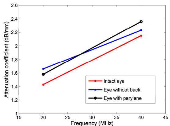
**Figure 5:** Comparison of the overall attenuation coefficient of different samples
