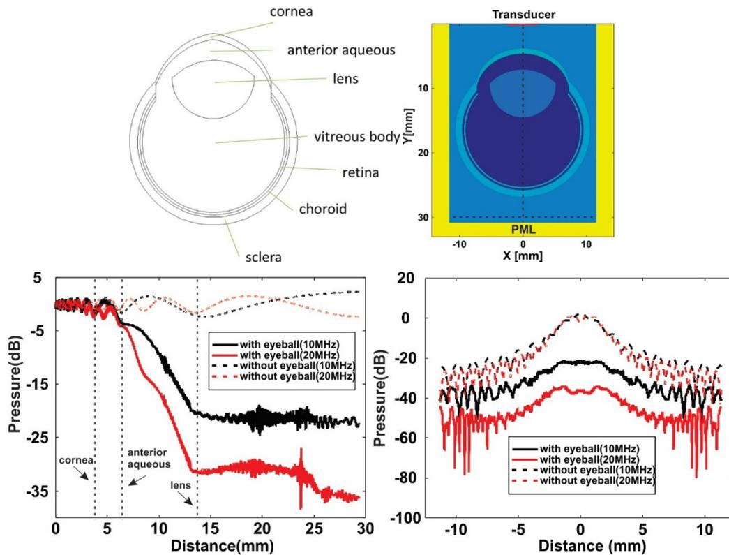
**Figure 3:** Two-dimensional simulated acoustic pressure profile in multilayered eyes at frequencies of 10-MHz and 20-MHz (a) Sketch of the porcine eye; (b) The structure of the eye for simulation; (c) Pressure profile along - y-direction; (d) Pressure profile along the x-direction.
