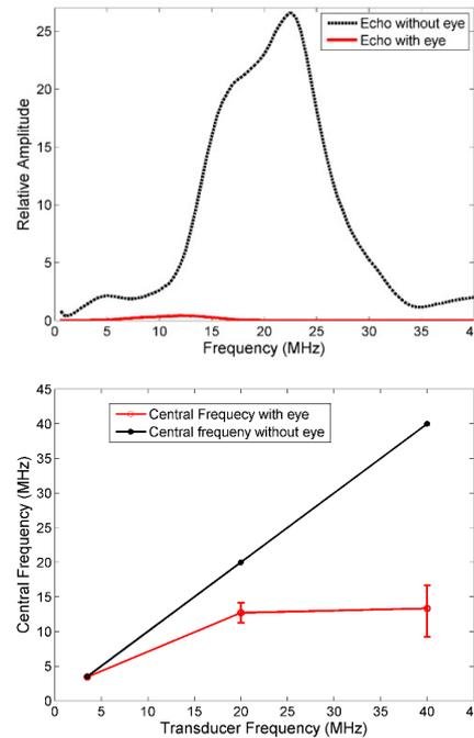
**Figure 2:** The central frequency shift after ultrasound penetration through porcine eyes. (a) Spectrum of the 3.5-MHz focused transducer; (b) Spectrum of the 20-MHz focused transducer; (c) Central frequency shift.
